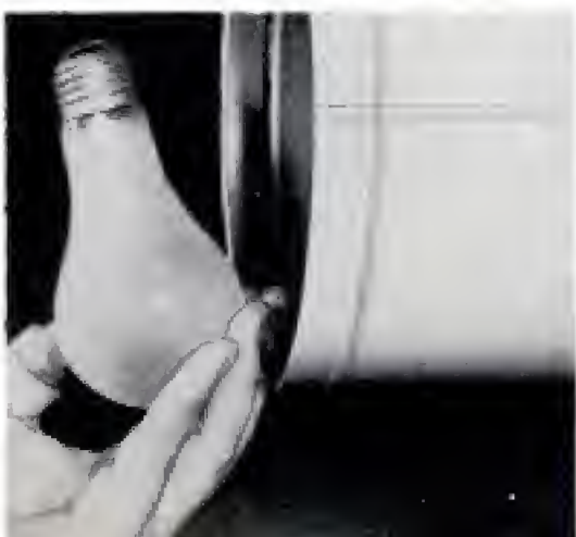
Lower left, No. 1 photoflood bulb gives ample light without excessive heat. Lower right, a hole about 3 in. in dia. in can lid gives fairly sharp spot. Can lid is removed when lamp is used for floodlighting
